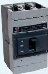
XB Frame : I cu /I cs = 25/25, 36/18, 36/36, 50/50 kA
